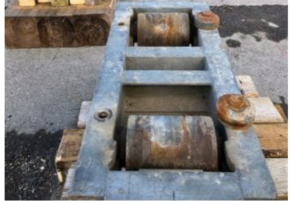
Roller system for cantilevered launch sequence.
